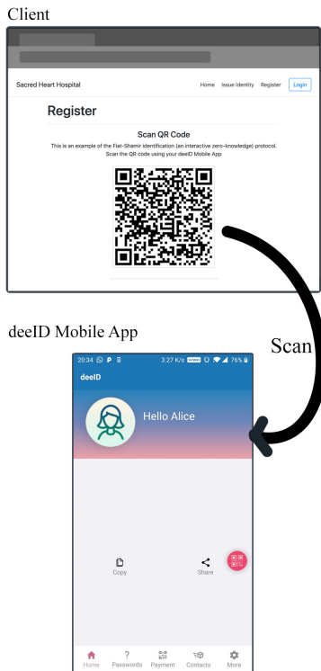
Figure 4: Client and mobile application interface design. Upon scanning the QR image the mobile application would recognise the message type and respond appropriately. In this instance it is an identification request.
