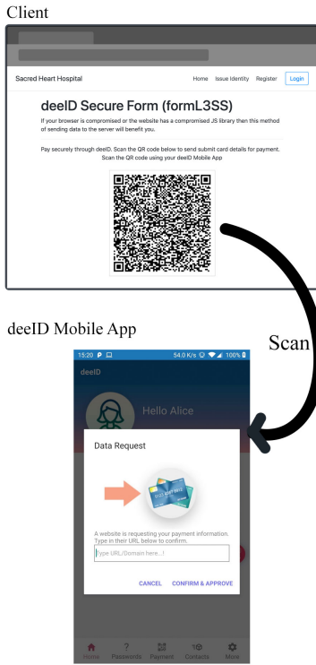
Fig. 3. Interface design of the web page and the mobile phone app. Upon scanning the image the mobile app will ensure the QR code's data is not manipulated by verifying the domain and its cryptographic signature.
